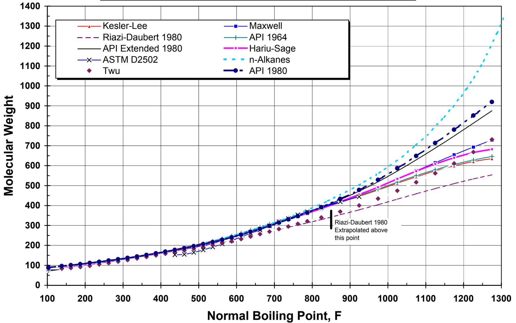
Figure 1A - North Slope Crude Molecular Weight Correlation Comparison - Expanded
